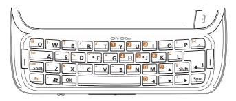
Your Acer M900 Smartphone has a key layout similar to your desktop or notebook computer for greater ease of use. Your Acer M900 Smartphone keyboard also has an embedded numeric keypad (highlighted in orange) for entering number data or dialing phone numbers.
