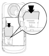
Place the battery into the battery compartment, lining up the battery connectors with those on the side the compartment.
