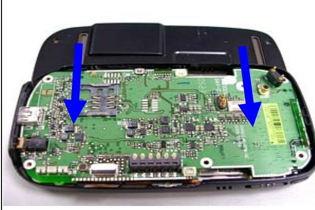
Shift the slide tray as left picture
