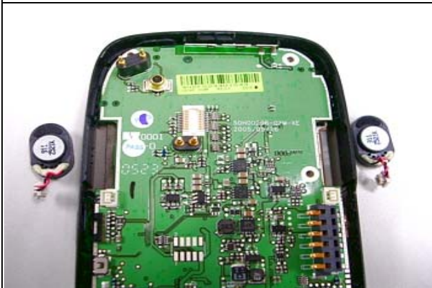
Both side speakers are removed
