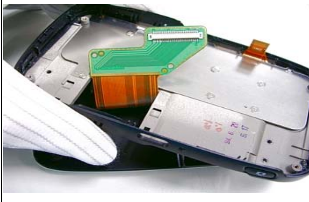
Assembly the tray of keyboard
