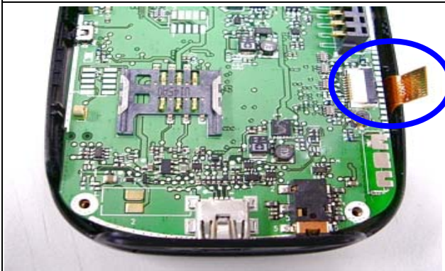
Disconnect keyboard FPC cable
