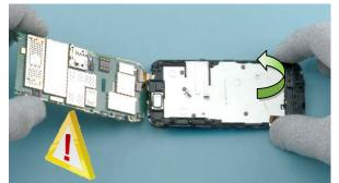
23) Turn over the ENGINE BOARD. Be careful not to break the flex!
