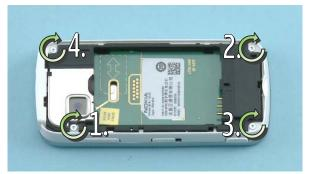
2) Tighten the screws to the torque of 17 Ncm in the order shown.
