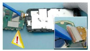
24) Open the locking mechanism of the LCD connector. Be careful not to damage the components nearby!
