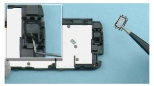
36) Remove it with the tweezers. Remove also the remains of the GASKET from the EAR PIECE.
