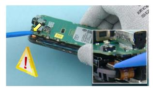
22) Also, open the UPPER FLEX ASSY connector on the top side of the phone with the SS-93. Be careful not to damage the components nearby!
