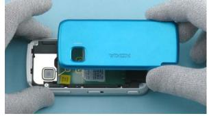
5) Remove the BATTERY COVER. If there is a battery inserted, remove it also.
