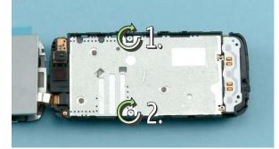
1) Tighten the 2 screws to the torque of 16 Ncm in the order shown.
