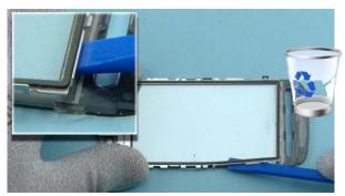
40) Use the SS-93 to detach the TOUCH FRAME ASSY from the TOUCH PANEL ASSY. TOUCH FRAME ASSY and TOUCH PANEL ASSY can now be separated. Do not use the TOUCH FRAME ASSY again. Discard it.
