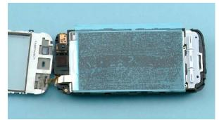
15) Protect the LCD with a protective film.
