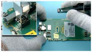
30) Use the camera removal tool SS-88 to lift up the camera.
