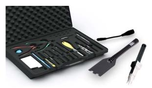
2) You must use the Nokia Standard Toolkit version 2. You will also need the SS-88 camera removal tool, SS-195 display removal tool and a DC plug.
