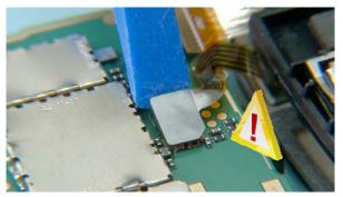
26) Open the TOUCH PANEL connector with the SS-93. Be careful not to damage the connector - or any nearby components!
