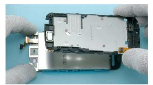
32) Remove the LCD FRAME ASSY.
