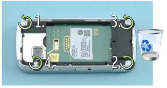
6) Unscrew the four TORX+ size 5 screws in the order shown. Remove them with the tweezers.
