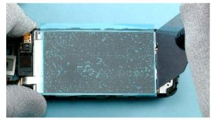
17) Insert the SS-195 display removal tool between the LCD and the LCD FRAME ASSY. Carefully slide the tool underneath the LCD to loosen the adhesive.
