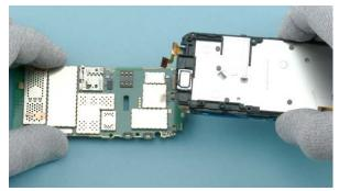
27) The engine board can now be separated.
