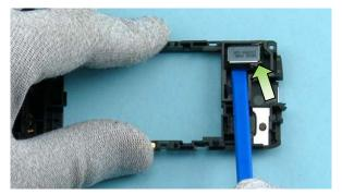
38) Lift up the IHF SPEAKER with the SS-93 and remove it using tweezers. Remains of the GASKET have to be removed from the IHF SPEAKER.
