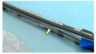
41) Also, make sure the adhesive which is on top of the TOUCH PANEL ASSY is removed while detaching the TOUCH FRAME ASSY.
