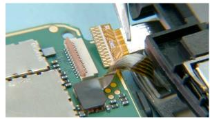
25) Release the LCD connector with the tweezers.
