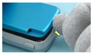
4) Use the opening notch to release the BATTERY COVER.
