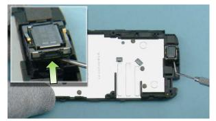
35) Lever out the EAR PIECE with the dental tool.
