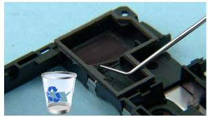
39) Peel out the corner of the IHF SPEAKER GASKET with the dental tool and remove it with tweezers. Do not use it again. Discard it.
