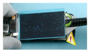
18) Lift up the bottom side of the LCD and then carefully lay it down. Be careful not to break the flex!
