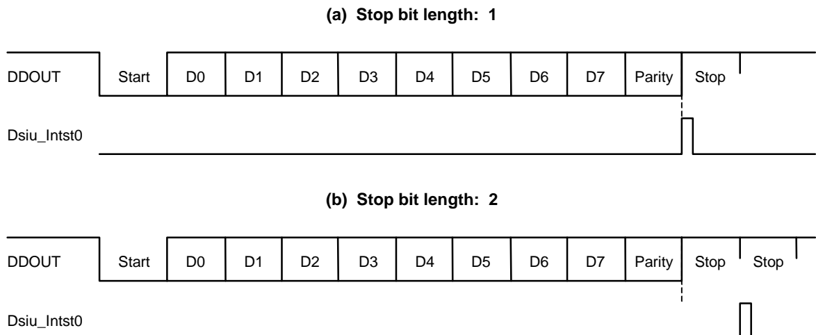
Figure 23-2. Transmit Complete Interrupt Timing
